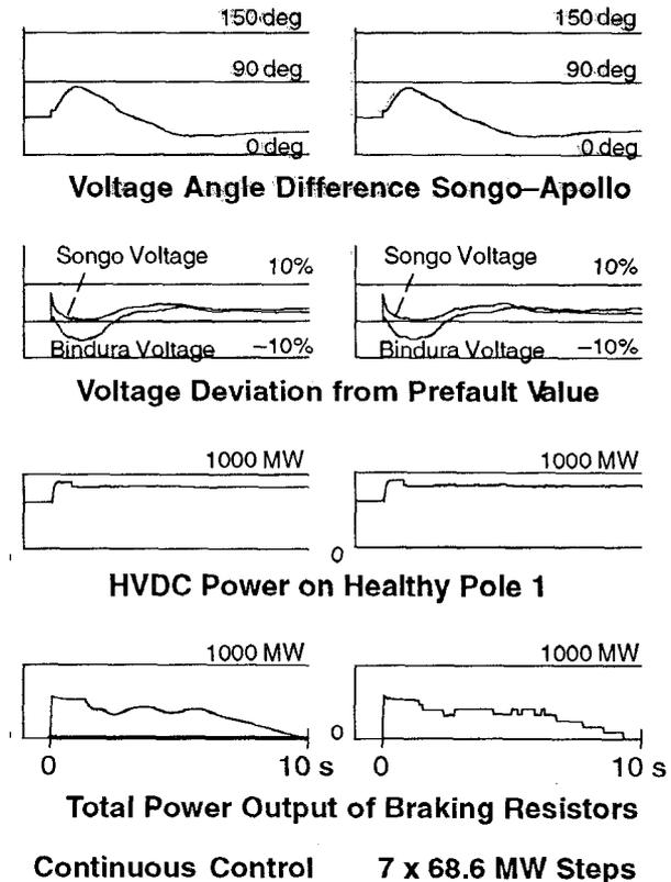
Fig. 3 : Comparison of Continuous or Stepwise Thyristor Control of Braking Resistors
