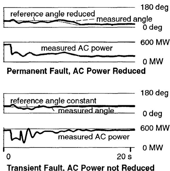
**Fig. 4 : AC Power Flow in the Bindura Line after a Fault in the Zimbabwe Network**
