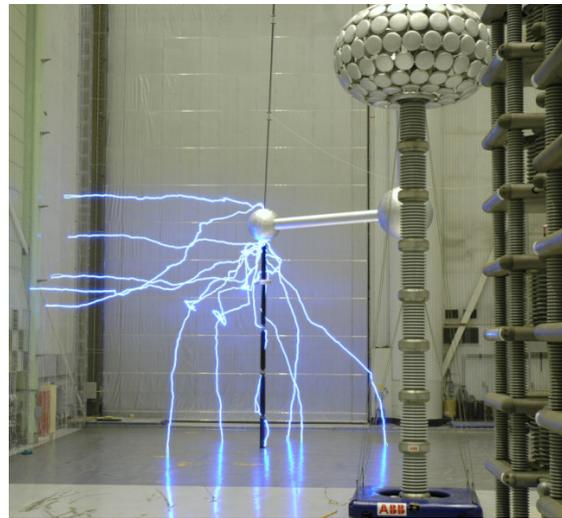
Fig. 6. Photograph of breakdown trajectories in a test set-up
