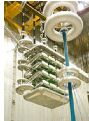
Fig. 9. A double valve for XS800 project at test position
