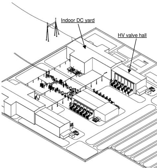
Fig. 2. Layout of converter station with indoor DC yard
